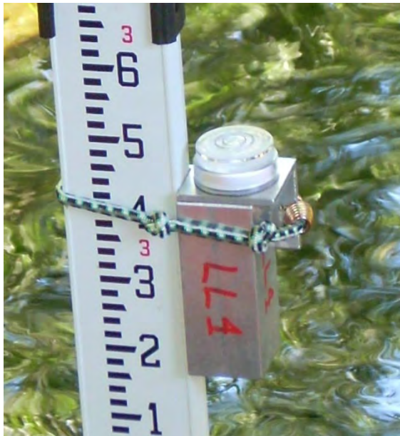
Figure 6 A circular bubble level is used to vertical the stadia rod. (Photo by Washington Dept. of Ecology)
