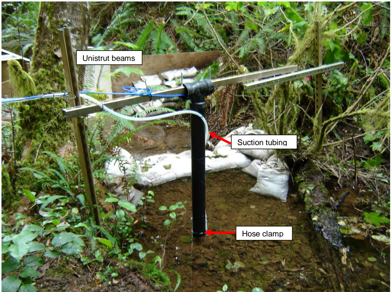
Figure 2. Turbidity sensor apparatus. The turbidity sensor is suspended inside the pipe and secured with hose clamps. The tee connector allows the pipe to move freely with the stream flow. Water is pumped from the stream through the suction tubing and into the pump sampler.
