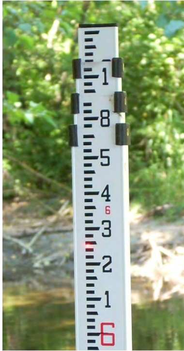
Figure 7 The center of the laser light dot projected on the rod is the point at which the stadia rod is read. (Photo by Washington Dept. of Ecology)
