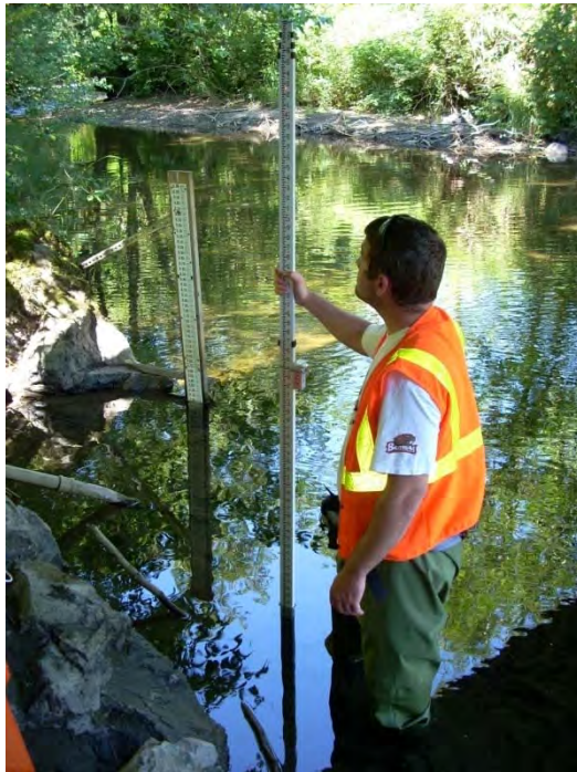
Figure 8 The rod is held perpendicular on solid substrate in calm water. (Photo by Washington Dept. of Ecology)
