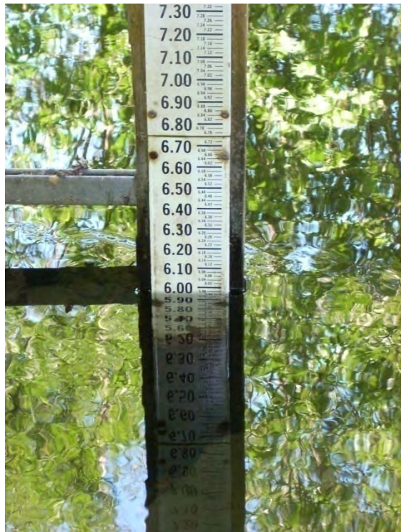
Figure 1 A typical Ecology staff gage with 0.02 feet increments. (Photo by Washington Dept. of Ecology)
