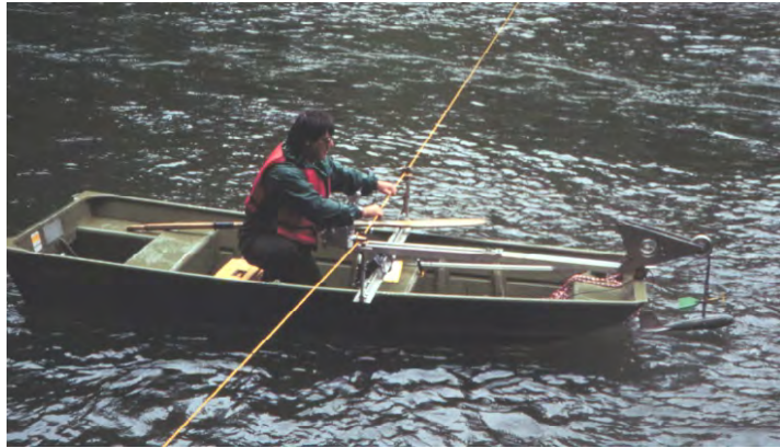
Figure 3 A boat measurement conducted with necessary equipment attached to a Kevlar® tag line. (Photo by Washington Dept. of Ecology)
