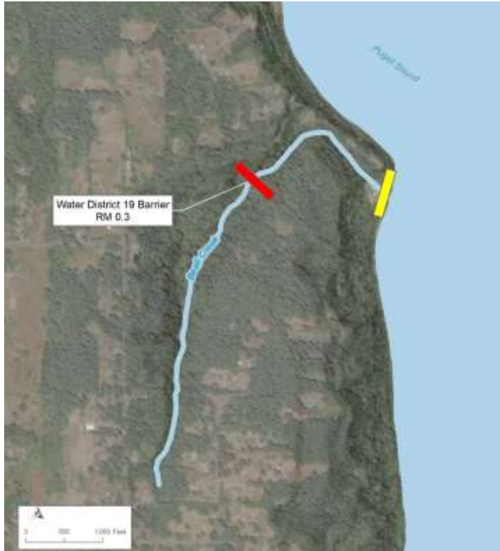
Figure 2. Beall Creek with a partial fish passage barrier at river mile 0.02 (yellow) and a complete fish passage barrier at river mile 0.30 (red). Both locations are associated with Water District 19. This project is focused on flow improvements at river mile 0.30.
